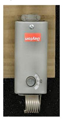
No, the picture is not upside down. Greenhouse thermostats that use a coil for improved accuracy are properly mounted with the coil portion down and in free air. This greatly improves sensitivity and also permits water sprayed or condensed on the coil to drain harmlessly away rather than expensively into the unit.
